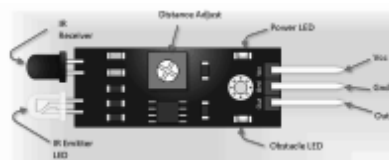
Fig.2 – Pin map of the FC-51 sensor.
