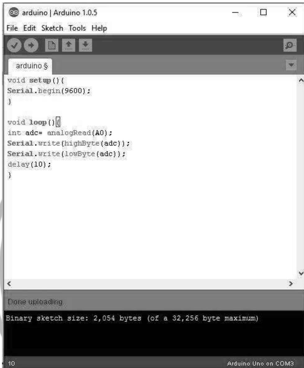
The image shows a screenshot of the Arduino IDE 1.0.5 software. The main window displays a C++ sketch for reading an analog sensor and sending data to the serial monitor. The sketch is as follows:
