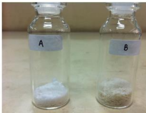
Fig. 1. Photographs of freeze-dried ovalbumin loaded alginate microspheres A: maltodextrin as lyoprotectant; B: lactose as lyoprotectant
