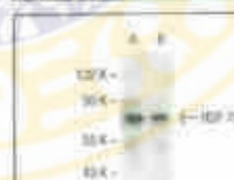
HSP 70 (F-3) (sc-373867) Western blot analysis of HSP 70 expression in HeLa (A) and NIH/3T3 (B) whole cell lysates.
