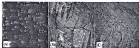
Figure 1: Crystal images obtained from polarization microscope with x100 magnification of Q (A), MA (B), and Q-MA (C) contact zones
