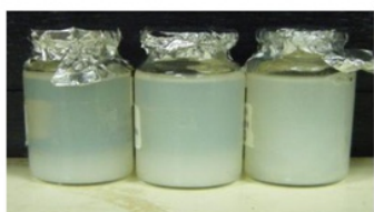
Fig. 4: Emulsion used VCO with surfactants-cosurfactants ratio of 4:1; 6:1; 7:1 and combination surfactants to produced HLB 12
