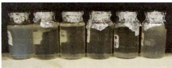
Fig. 5: Emulsions used VCO with surfactants-cosurfactants ratio of 3:1; 4:1; 5:1; 6:1; 7:1; 8:1 and surfactants combination to produced HLB 13
