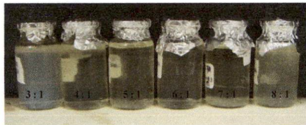
Fig.5; Emulsions used VCO with surfactants-cosurfactants ratio of 3:1; 4:1; 5:1; 6:1; 7:1; 8:1 and surfactants combination to produced HLB 13
