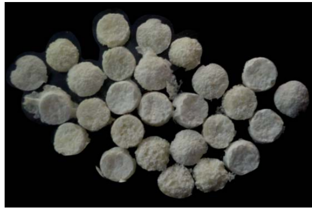
Fig. 1. Result of scaffolds making process using freeze dry method
