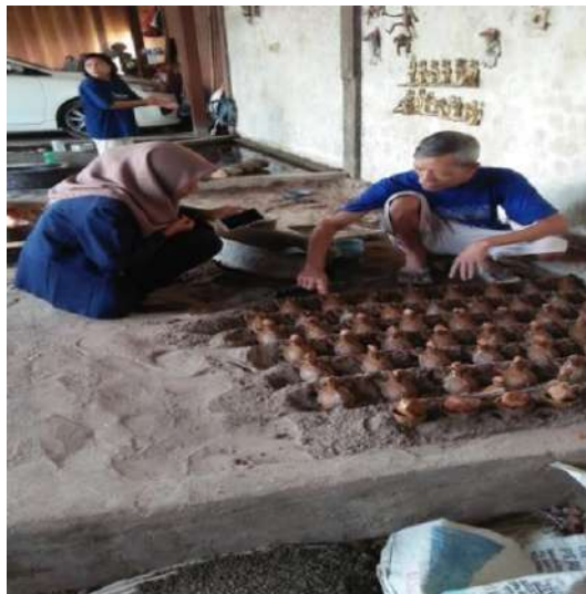
Gambar 2.27. Proses pengisian tanah/ Naceli
