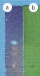
Figure 1. Thin layer chromatography of Spilanthes acmella auct. non (L) murray aerial part. a. observed in UV light 366 nm; b. observed in UV light 254 nm
