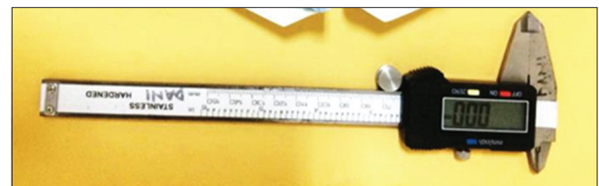
Figure 1: Digital vernier caliper with 0.01 least count (Gauge Block No. 020048)
