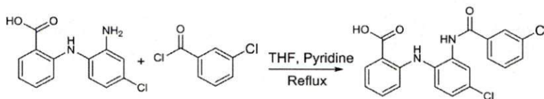
Figure 3: Synthesis of 3-Chlorobenzoyl-N-(2-amino-4-chlorophenyl) anthranilic Acid
