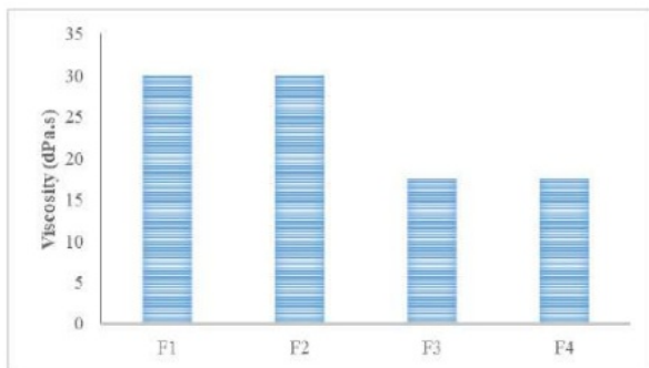
Figure 2: Viscosity evaluation results from carboxymethyl chitosan-curcumin hydrogel F I, F II, F III, and F IV.
