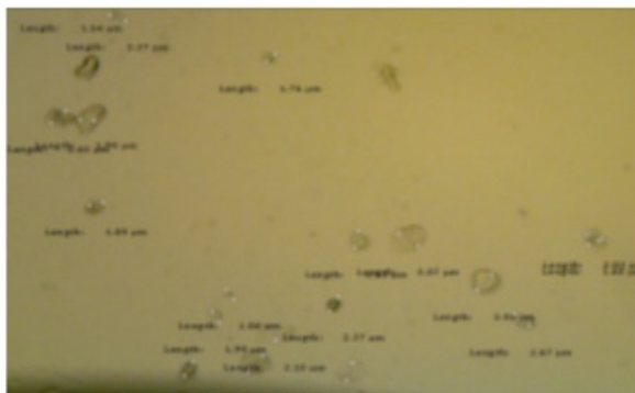
Figure 2: The results of the examination of particle shape of gentamicin sulfate dry microspheres using Biological Microscope Model XSZ-107 Series with 400x magnification.
