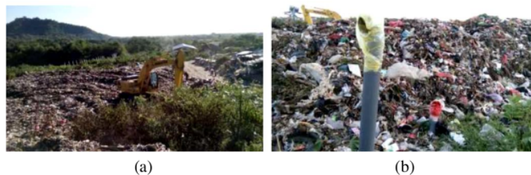
Figure 2. (a) Cell 3 condition at Klotok I Landfill with newly accumulated waste and (b) the height of waste pile during the measurement of CH 4 gas in Cell 3.
