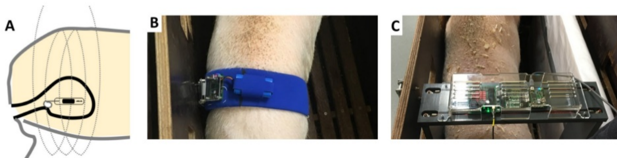
Fig 2. Principle of Bladder Pill for pressure measurement in animals. (A) Diagram of working mechanism of Bladder Pill in vivo, wireless induction as represented by coils (dotted lines) contained within a corresponding external device. (B) Waistband-form external device tested in vivo. (C) Rectangular frame. https://doi.org/10.1371/journal.pone.0225821.g002
